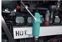
Ölabsaugpumpe Oil drain pump
