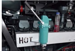
Ölabsaugpumpe Oil drain pump
